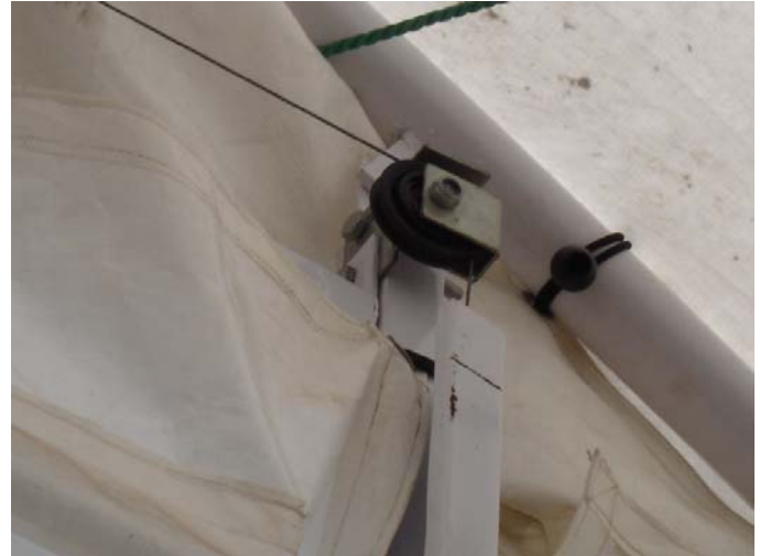
Single Door Pulley Farthest From Winch Assembly
