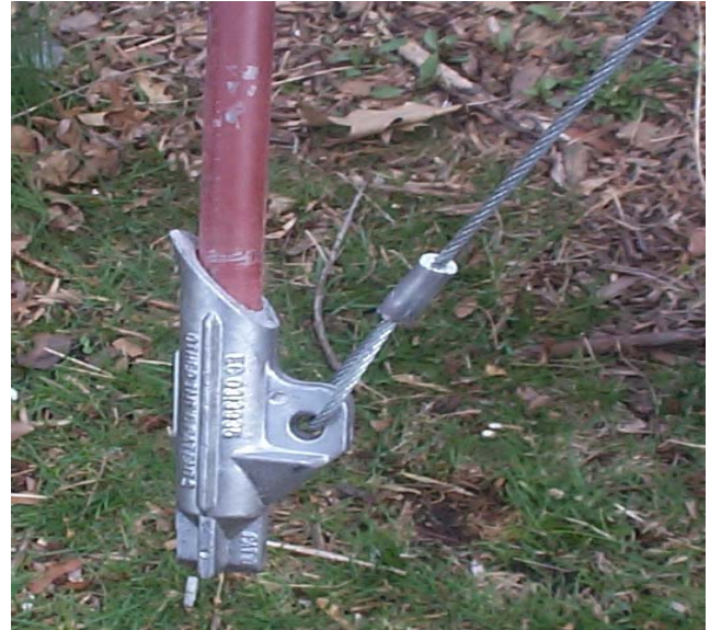
Drive Rod inserts into Anchor Head
